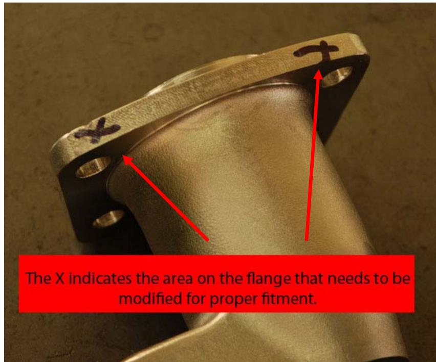
The X indicates the area on the flange that needs to be modified for proper fitment.
